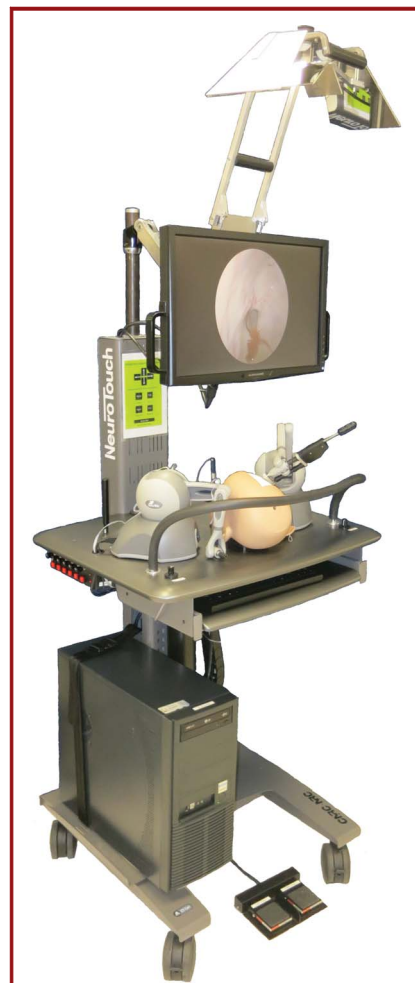
FIGURE 1. NeuroTouch, the National Research Council Canada's virtual reality simulator. The system was designed for neurosurgical resident training with exercises ranging from basic instrument handling of commonly used instruments to realistic neuro-oncology procedures for both open cranial and endoscopic interventions. The simulator in endonasal configuration is shown.
