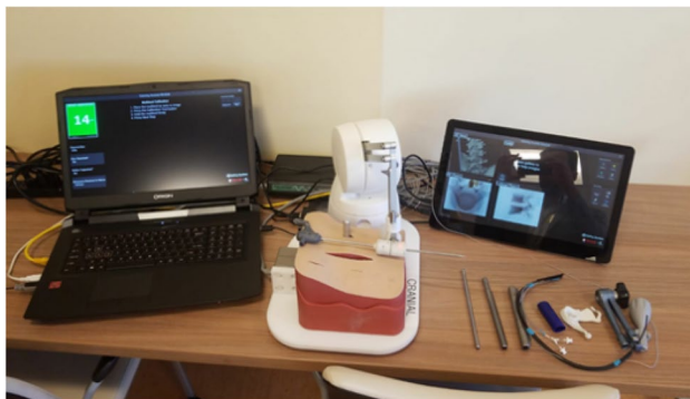
Fig. 1 The summarized simulator layout. Left is the laptop runs 120 Hz display, which indicates the instruction of the surgery process. The haptic device and benchtop model are in the middle. And right is the external display runs 60 Hz which indicates the four cameras that demonstrate the surgical area. The surgeon operates the haptic device based on the visual feedback from both monitors
