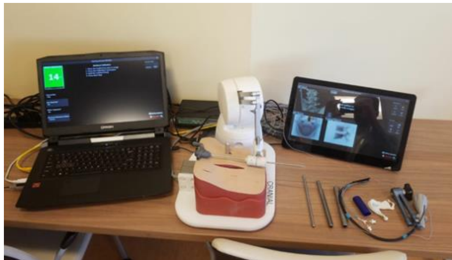
Figure 3-1 The summarized simulator layout. Left is the laptop runs 120Hz display, which indicates the instruction of the surgery process. The haptic device and benchtop model are in the middle. And right is the external display runs 60Hz which indicates the four cameras that demonstrate the surgical area. The surgeon operates the haptic device based on the visual feedback from both monitors.
