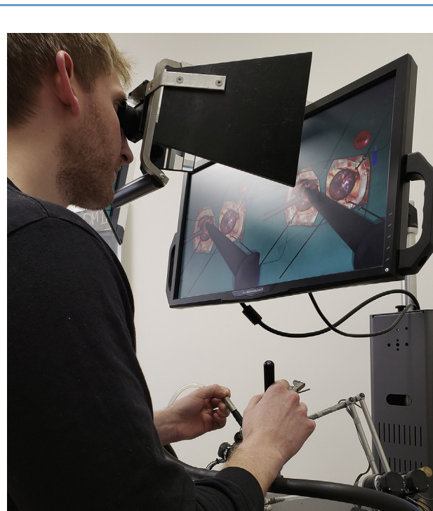
Figure 1. One of the authors performs a simulated brain tumor resection task on the NeuroVR neurosurgical simulation platform.
